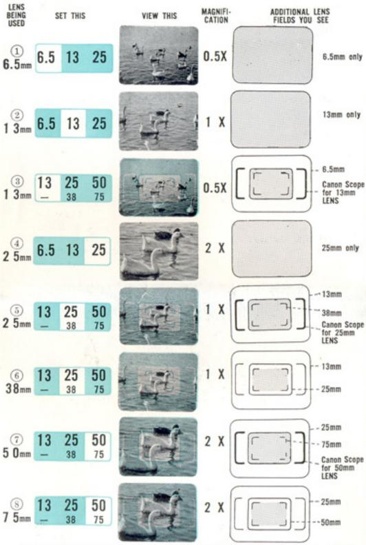
Note: Both 13mm and 25mm lenses can be viewed in two positions, either full frame, or as a brightly framed sports type finder. Note also that each focal length is provided with a 1:1 life size image for two-eye focusing. When using 13, 25, 38, 50 and 75mm lenses, brightly framed sports type finder enables the easy composition and perfect timing as the object moves into the picture area.
