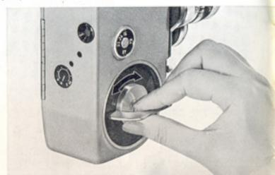
To open the SIDE COVER, lift up the OPENING KEY and turn it to the left. The moment the SIDE COVER is opened, the PRESSURE PAD of the FILM GATE will automatically be released and the FOOTAGE COUNTER reset to "S" (starting position).
