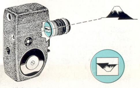
idle lenses. Focus as described above. Return the taking lens to the original position.
