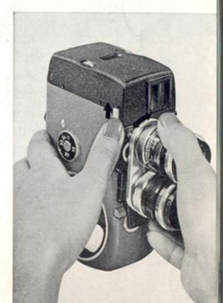
When your camera is in focus for a certain object, it is also in focus for a range of objects in front and behind that object. This range is called the Depth-of-Field and shown on your lens—the DEPTH-OF-FIELD SCALE. You can also know it sighting through the FOCUSING FINDER (in case of Canon Eight "T").
