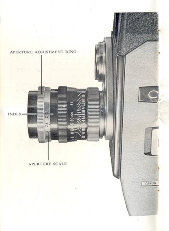
The diaphragm of the lens is designed to control the amount of light which passes it and reaches the film. The APERTURE ADJUSTMENT RING of your Canon Cine Lens enables you to alter the aperture of the diaphragm and control the light amount.
