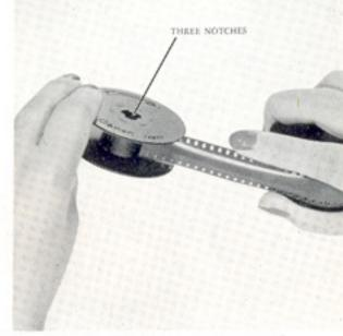
Then, wind at least two or three turns of film onto the spool.
