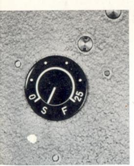
the film exposed just by a glance on the FOOTAGE COUNTER. Every time 6 inches of film is exposed, you will also hear a click. This will enable you to check on the length of a scene. Each full winding of the motor allows you to shoot 5 feet of film, at any speed.
