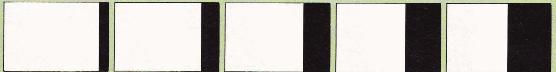
MAA 511 HORIZONTAL WIPE expands from 3 - 33mm in 3mm increments
